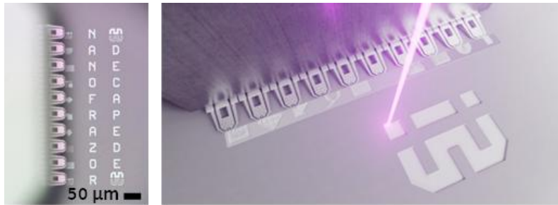
Figure 1: (left) NanoFrazor in-situ microscope showing the Decapede over a resist-coated substrate, writing features in both 2D high-resolution and in grayscale. (right) Simulated image of the Decapede patterning different features, alongside the integrated laser writehead.
