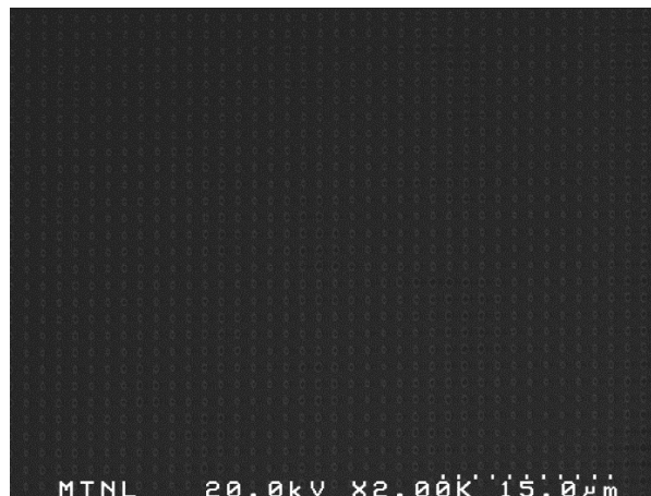
Figure 3: Top-down image of patterned photoresist pillars on silicon wafer at 2kX magnification.
